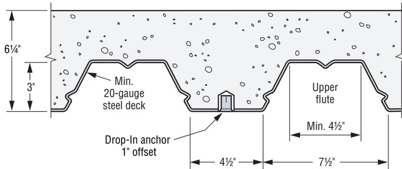
Figure 1. Lightweight Concrete over Steel Deck
