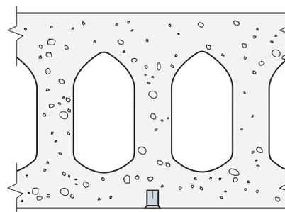
Figure 2. Hollow-Core Concrete Panel
